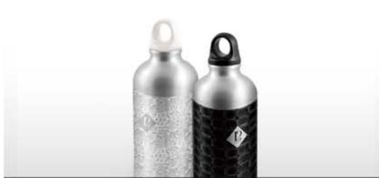
Using an optional rotary axis fixture, print graphics onto bottles and other cylindrical items.
