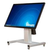
Motorized stands allow for unprecedented versatility and convert a touch display from a touch wall to a multitouch table or even a drafting-style orientation. (Not available for the 86" model.)
