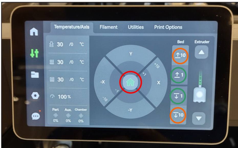
Control Panel on the X1E
